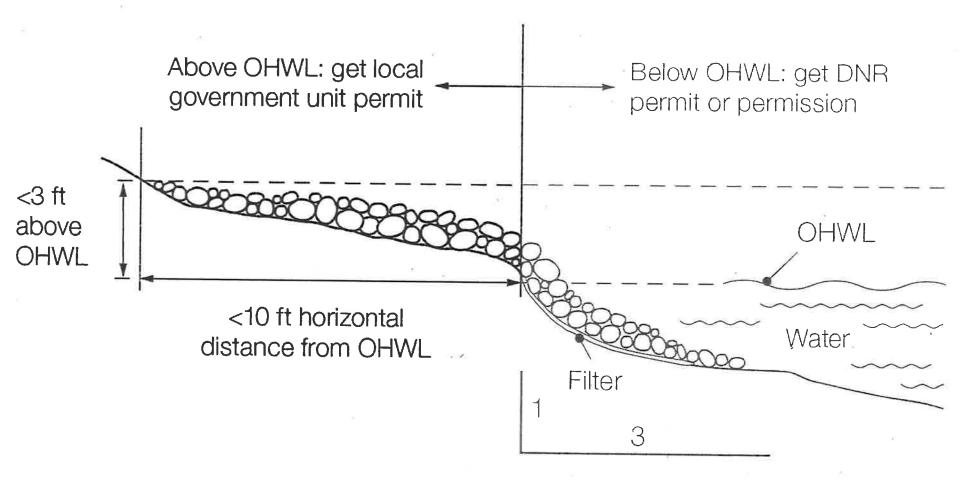
Finished slope below OHWL must be less than a 1:3 ratio
