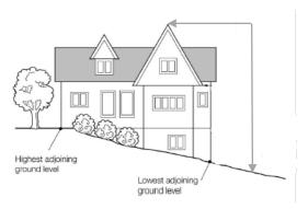
Structure height: The vertical distance between the lowest adjoining ground level at the building and the highest point of the roof.
