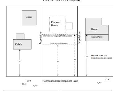
Averaging Setbacks:  $78^{\circ}+42^{\circ}=120^{\circ}\div2=60^{\circ}$ Add  $20^{\circ}$  to Average:  $60^{\circ}+20^{\circ}=80^{\circ}$ In this example Shoreline Averaging  $=80^{\circ}$ (Minimum setback is the Shore Impact Zone Line)
