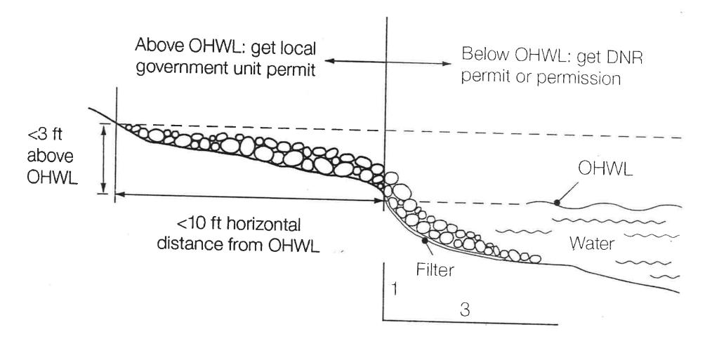
Finished slope below OHWL must be less than a 1:3 ratio
