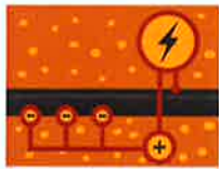
Maintaining cathodic protection (an electrical current that curbs corrosion)
