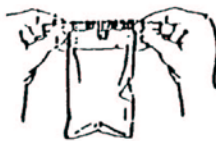
E. Straighten wires by pulling on the ends of the wire.
