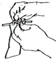
B. Separate the wires by pulling the tabs outward.
